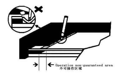
**b.** Since ITO of film and glass is not eliminated at the edge, therefore please design as any conductive material does not touch the edge of touch panel.
