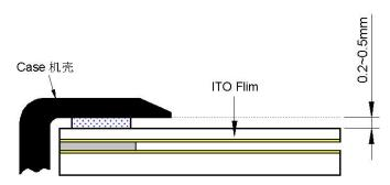
5) We recommend to design a case that it covers the boundary of the active area inside in order to prevent an operation at outside of the active area which can not guarantee the specified durability, because operation at the outside of the active area causes serious damage of a transparent electrode.
