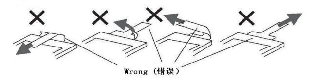
Do not fix, adhere or mount any additional goods on the FPC such as additional film/plate on the FPC as shown in below, because such additional goods emphasizes a stress applied at the tip of FPC and it works tearing off the root of FPC from touch panel.
