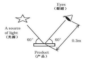
Visual inspection shall be done at a distance of 0.3 m between eyes and a product with an angles of  $60^{\circ} \pm 10^{\circ}$  to the surface of the product under a ceiling fluorescent light (40 W, natural color). An environmental condition for judge is at 23 °C  $\pm 5$  °C,55 %RH $\pm 10$  %RH and 860 h Pa to 1060 h Pa. This standard shall be applied to the initial status.
