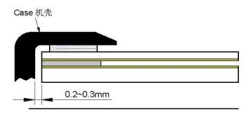
Meanwhile, in order to avoid touch panel any failure for extra wrap tail, please take care of keeping clearance of 2.0min.between tail position and inside boundary of case when the touch panel is built into case.
