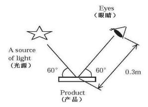
Visual inspection shall be done at a distance of 0.3 m between eyes and a product with an angles of  $60^{\circ} \pm 10^{\circ}$  to the surface of the product under a ceiling fluorescent light (40 W, natural color).An environmental condition for judge is at 23 °C ±5 °C,55 %RH±10 %RH and 860 h Pa to 1060 h Pa. This standard shall be applied to the initial status.
