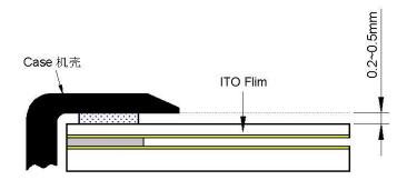
5) We recommend to design a case that it covers the boundary of the active area inside in order to prevent an operation at outside of the active area which can not guarantee the specified durability, because operation at the outside of the active area causes serious damage of a transparent electrode.
