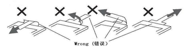
Do not fix, adhere or mount any additional goods on the FPC such as additional film/plate on the FPC as shown in below, because such additional goods emphasizes a stress applied at the tip of FPC and it works tearing off the root of FPC from touch panel.
