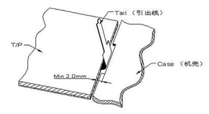
8) Please keep your case flat in order not to touch with touch panel directly, which causes serious damage of a transparent electrode.
