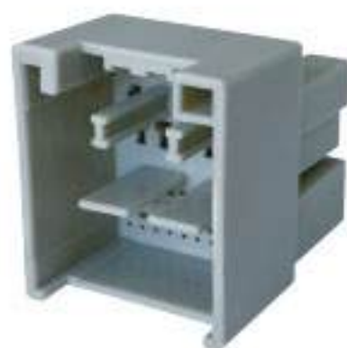
Type: TS30284-32P-11-1 Material: PA66 GF30% Matching Terminal: TSZ024 / TSZ144 / TSZ208B
