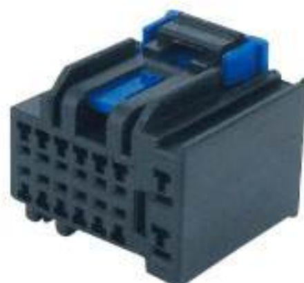
Type: TS2105-14P-21-1 Material: PA66 GF30% Matching Terminal: TSH006/TSH009
