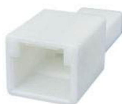
Type: TS30163-03P-11 Material: PA66 Matching Terminal: TSZ208
