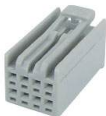
Type: TS1730-08P-21 Material: PA66 Matching Terminal: TSH143
