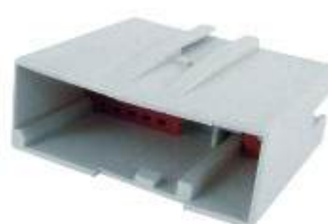
Type: TS5520-24P-11 Material: PA66 GF30% Matching Terminal: TSZ143 / TSZ144 / TSZ145
