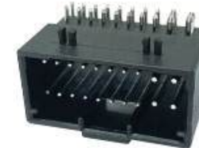
Type: TS30322-20PM-PKB Material: PA66 GF30% Matching Terminal: TSPM0104A / TSPM0107A / TSPM0167~TSPM0168
