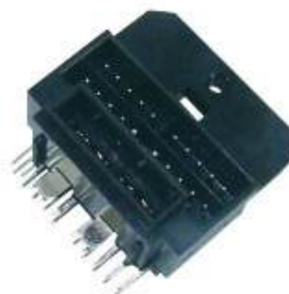
Type: TSJEN-20PM-PKB-2 Material: PBT GF30% Matching Terminal: TSPM0099~TSPM0102
