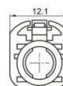
Type: TSVW20-04PF-AT-5LG Material: PA66 GF30% Matching Terminal: TSTF0048 / TSTF0049 / TSTF0050
