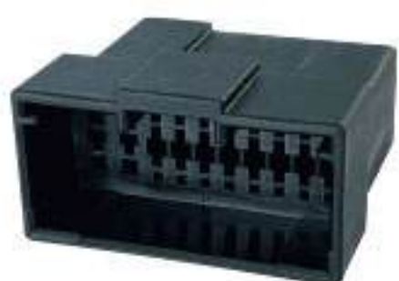
Type: TS30322-20P-11 Material: PA66 GF30% Matching Terminal: TSZ032 / TSZ031
