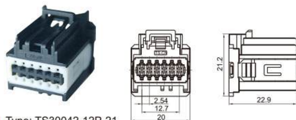
Type: TS30042-12P-21 Material: PA66 GF30% Matching Terminal: TSH006
