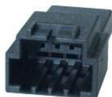
Type: TS30150-04P-11 Material: PA66 GF30% Matching Terminal: TSZ208
