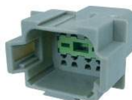
Type: TS30267-08P-11 Material: PBT GF15% Matching Terminal: TSZ621
