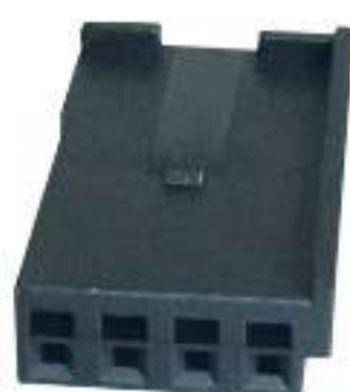
Type: TSBM04-04P-21-4 Material: PA66 GF15% Matching Terminal: TSH143
