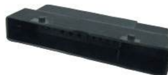
Type: TSAD32-32P-11 Material: PA66 GF30% Matching Terminal: TSZ028 / TSZ024 / TSZ040
