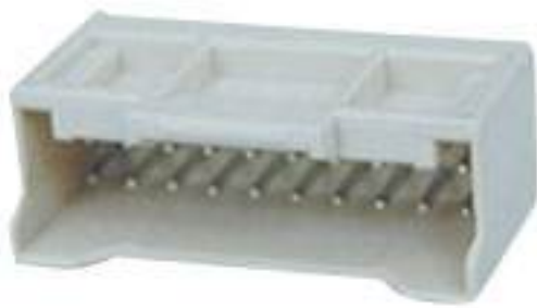
Type: TS30046-20PM-PKS(QRA3) Material: PA66 GF15% Matching Terminal: TSPM0145
