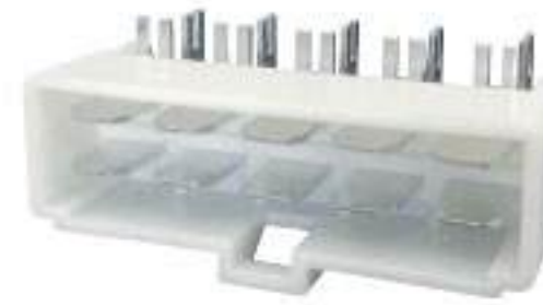
Type: TS30198-10PM-PKB Material: PA66 GF30% Matching Terminal: TSPM0308 / TSPM0309
