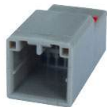
Type: TS6502-10P-11-1 Material: PA66 Matching Terminal: TSZ553
