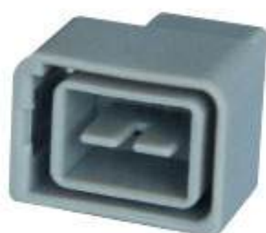
Type: TSNI10-10P-11 Material: PA66 GF30% Matching Terminal: TSZ540 / TSZ537
