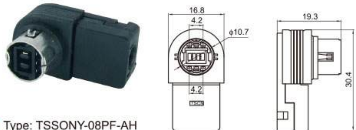
Type: TSSONY-08PM-AH Material: PA66 GF30% Matching Terminal: TSAM0001 / TSAM0003 / TSAM0002
