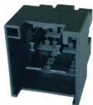
Type: TS30284-32P-11 Material: PA66 GF30% Matching Terminal: TSZ024 / TSZ144 / TSZ208B
