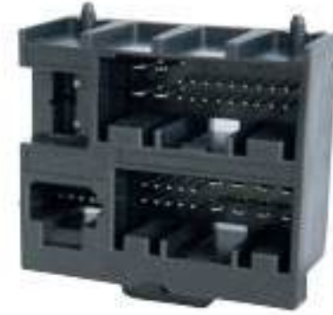
Type: TS30051-52PM-PKS Material: PA66 GF30% Matching Terminal: TSPM0121 / TSPM0207~TSPM0210
