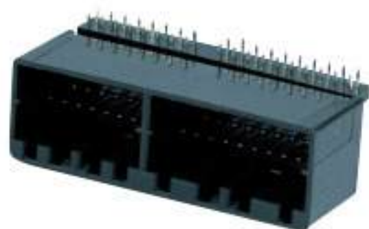
Type: TSHD36-36PM-PKB-2 Material: PA66 Matching Terminal: TSPM0088 / TSPM0089
