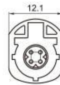
Type: TSVW10-04PM-AT-5BK Material: PA66 GF30% Matching Terminal: TSPM0021~TSPM0025
