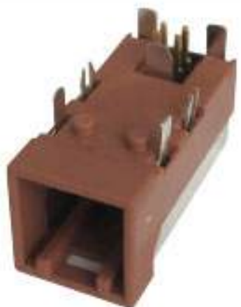
Type: TSTA04-04PM-AT-PKB-2 Material: PBT GF15% Matching Terminal: TSPM0050 / TSPM0053
