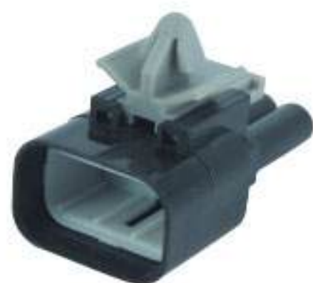
Type: TS3012-03P-11 Material: PA66 Matching Terminal: TSZ011
