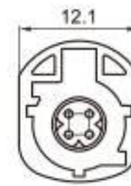
Type: TSVW10-04PM-AT-5BE Material: PA66 GF30% Matching Terminal: TSPM0021~TSPM0025
