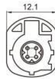
Type: TSVW10-04PM-AT-5BN Material: PA66 GF30% Matching Terminal: TSPM0021~TSPM0025
