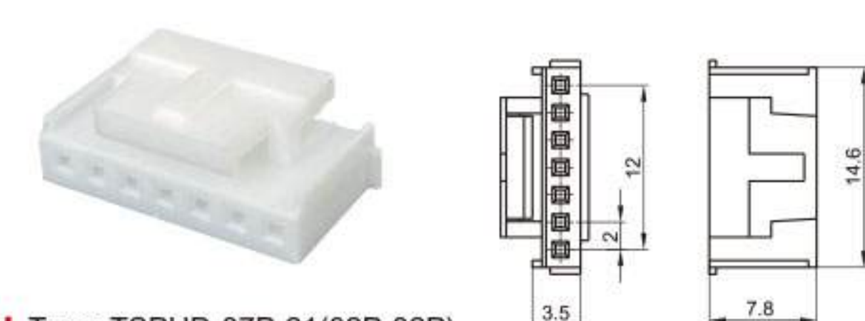
Type: TSPHD-07P-21(02P-32P) Material: PA66 Matching Terminal: TSPHD
