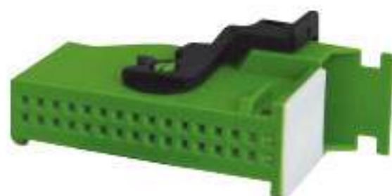
Type: TSAD32-32P-21-2 Material: PA66 Matching Terminal: TSH092
