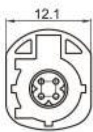
Type: TSVW10-04PM-AT-5GN Material: PA66 GF30% Matching Terminal: TSPM0021~TSPM0025
