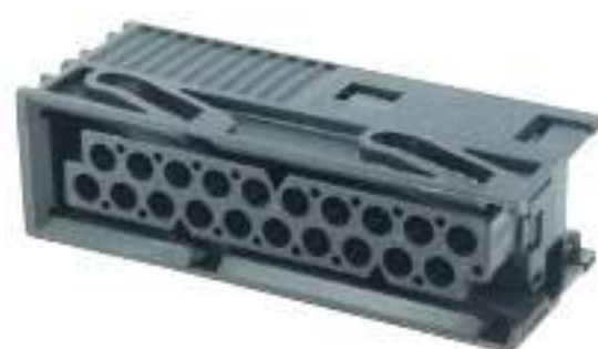
Type: TSBM20-20P-21 Material: PA66 GF30% Matching Terminal: TSH078
