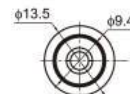
Type: TSAF-AT Material: PA66 Matching Terminal: TSTF0012 / TSTF0013
