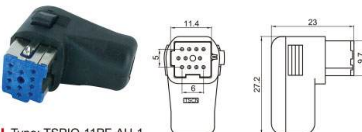
Type: TSPIO-11PF-AH-1 Material: PA66 GF30% Matching Terminal: TSAF0009 / TSAF0010 / TSH501
