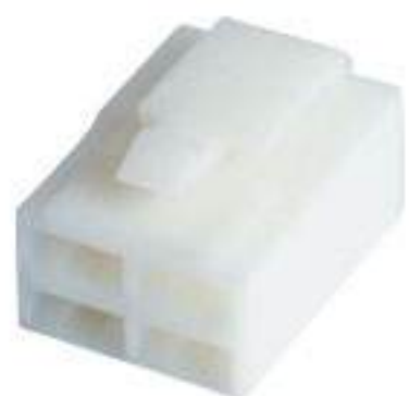
Type: TS1781-04P-21 Material: PA66 Matching Terminal: TSH607
