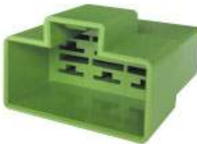
Type: TS30002-06P-11-1 Material: PBT GF15% Matching Terminal: TSZ538-A
