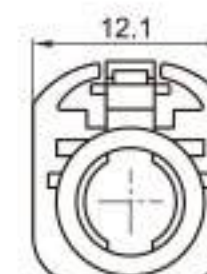
Type: TSVW20-04PF-AT-5GY Material: PA66 GF30% Matching Terminal: TSTF0048 / TSTF0049 / TSTF0050
