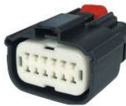
Type: TS30359-12P-21 Material: PA66 GF30% Matching Terminal: TSH047
