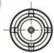
Type: TSFIAT10-01PM-AT Material: PA66 GF30% Matching Terminal: TSTM0012/TSTM0013
