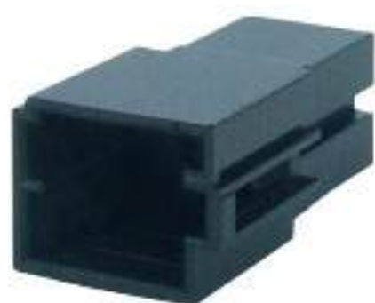
Type: TSVW08-08P-11 Material: PA66 Matching Terminal: TSZ040
