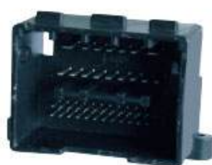
Type: TSKL44-44PM-PKS Material: PA66 GF30% Matching Terminal: NIL
