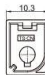
Type: TS1068-01PM-AT-2 Material: PA66 Matching Terminal: TSTM0003 / TSTM0004
