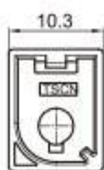
Type: TS1068-01PM-AT Material: PA66 GF30% Matching Terminal: TSTM0003 / TSTM0004
