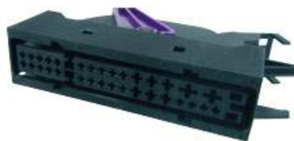
Type: TSAD32-32P-21 Material: PA66 GF30% Matching Terminal: TSH019E / TSH019 / TSH054
