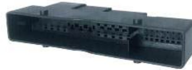
Type: TS30282-38P-11 Material: PBT GF15% Matching Terminal: TSZ028 / TSZ024 / TSZ040 / TSZ208
