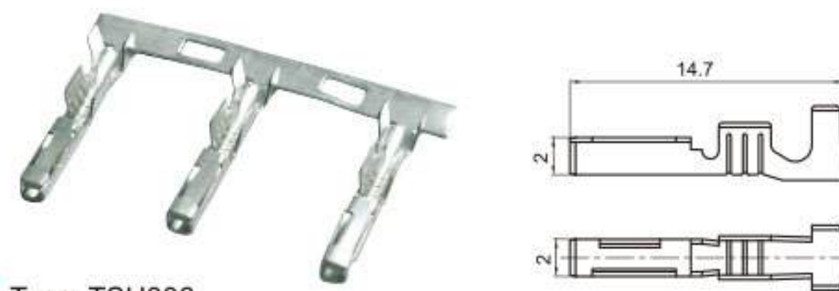
Type: TSH006 Material: Phos.bronze Applicable Thickness: 0.6
