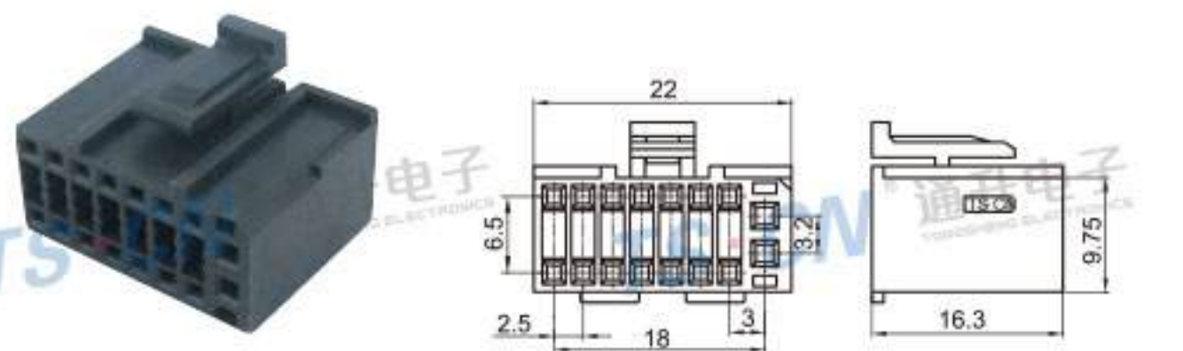
Type: TSDR16-16P-21 Material: PA66 GF30% Matching Terminal: TSVH / TSH118
