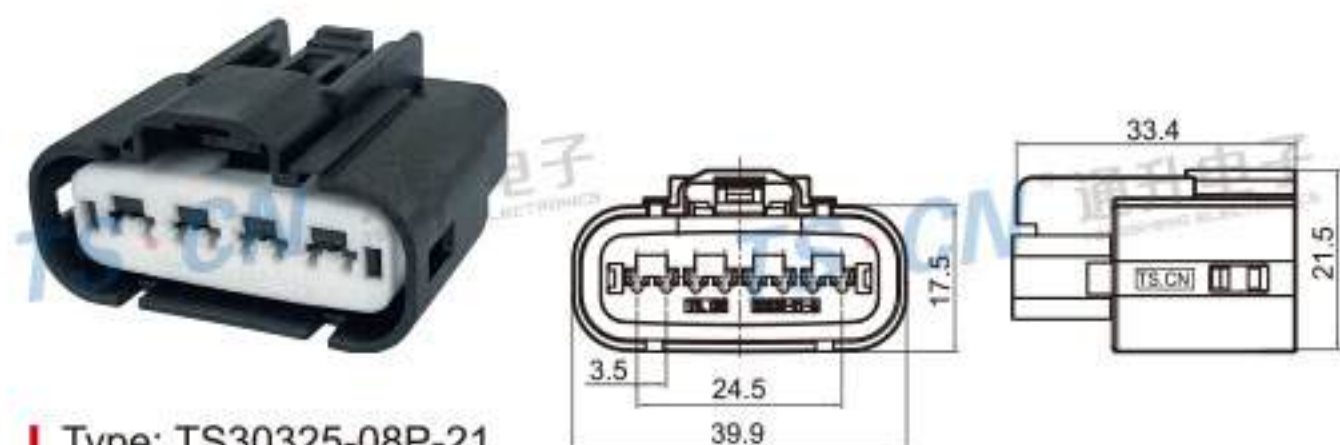
Type: TS30325-08P-21 Material: PBT Matching Terminal: TSH047
