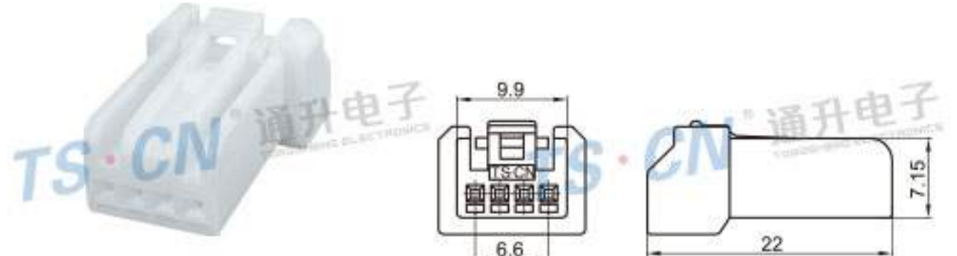
Type: TS30203-04P-21 Material: PA66 Matching Terminal: TSH143
