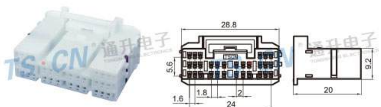
Type: TS30101-30P-21-4 Material: PA66 Matching Terminal: TSH600A
