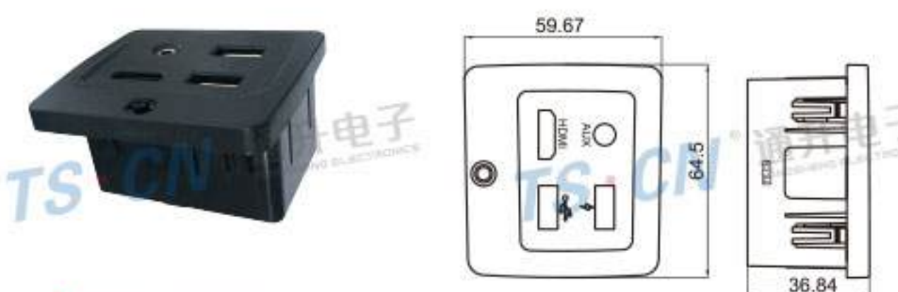
Type: TS30252 Material: ABS Matching Terminal: TSHDMI-F / TSUSB-F / TS3.5-F
