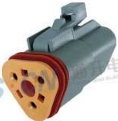
Type: TS30267-03P-21 Material: PBT GF15% Matching Terminal: TSH646
