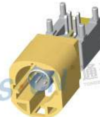
Type: TSVW10-04PM-AT-5BE Material: PA66 GF30% Matching Terminal: TSPM0021~TSPM0025
