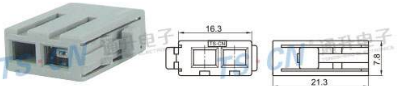
Type: TSK120-02PF-AT Material: PA66 Matching Terminal: TSTF0001 / TSTF0002
