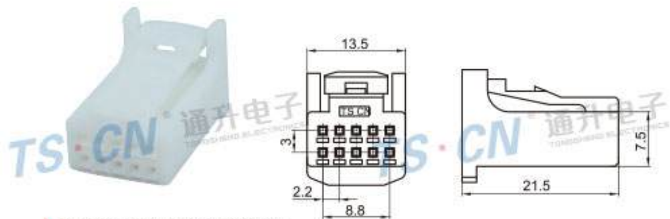
Type: TSTA10-10P-21-1 Material: PA66 Matching Terminal: TSH143
