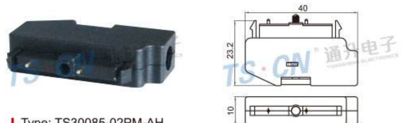
Type: TS30085-02PM-AH Material: PA66 Matching Terminal: TSAM0023 / TSAM0024
