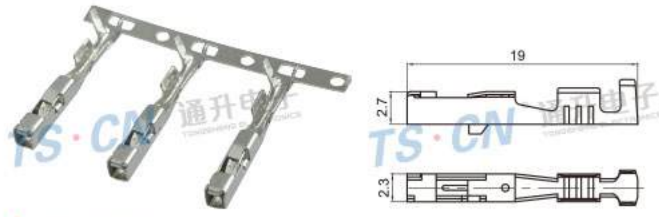
Type: TSH008 Material: Phos.bronze Applicable Thickness: 0.6~0.8
