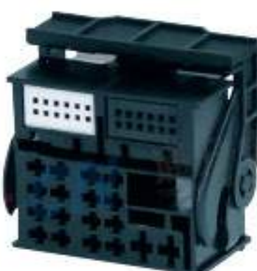
Type: TS9003-42P-21-6 Material: PA66 GF30% Matching Terminal: TSH019E / TSH019 / TSH143
