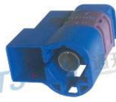
Type: TSVW10-08PM-AT-1BL Material: PBT GF15% Matching Terminal: TSPM0175 / TSTM0051 / TSZ208
