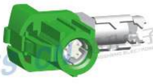
Type: TSVW20-04PF-AT-5GN Material: PA66 GF30% Matching Terminal: TSTF0048 / TSTF0049 / TSTF0050
