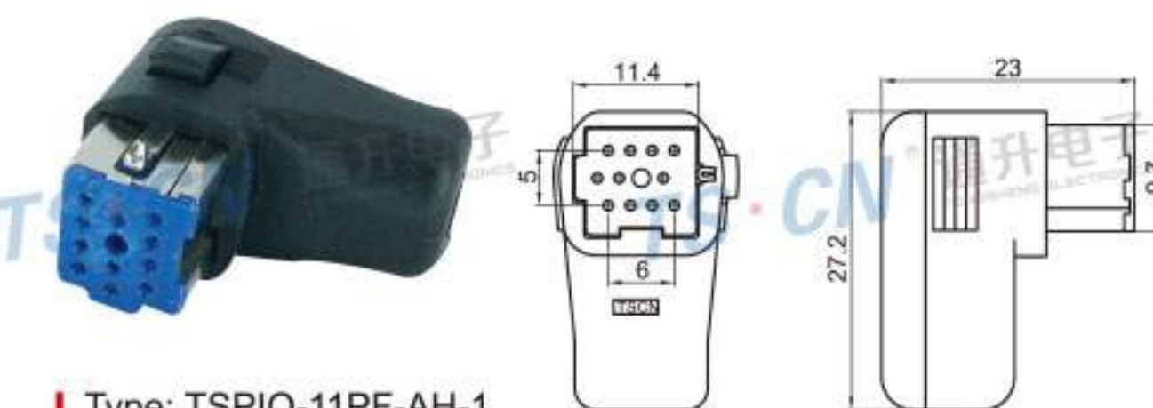
Type: TSPIO-11PF-AH-1 Material: PA66 GF30% Matching Terminal: TSAF0009 / TSAF0010 / TSH501
