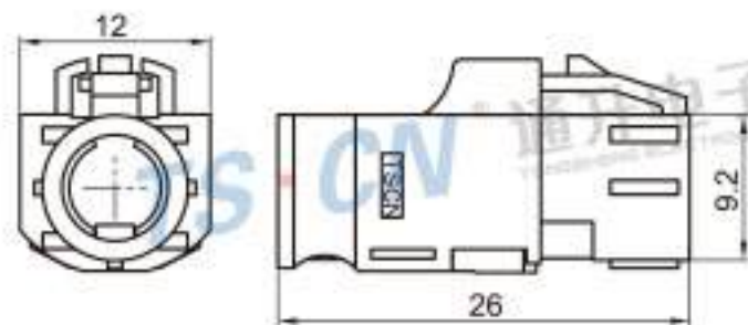
Type: TSVW20-04PF-AT-5WB-1 Material: PA66 GF30% Matching Terminal: TSTF0051 / TSTF0052
