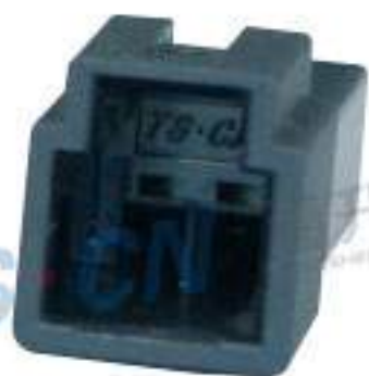
Type: TS30117-02P-11 Material: PA66 Matching Terminal: TSZ145
