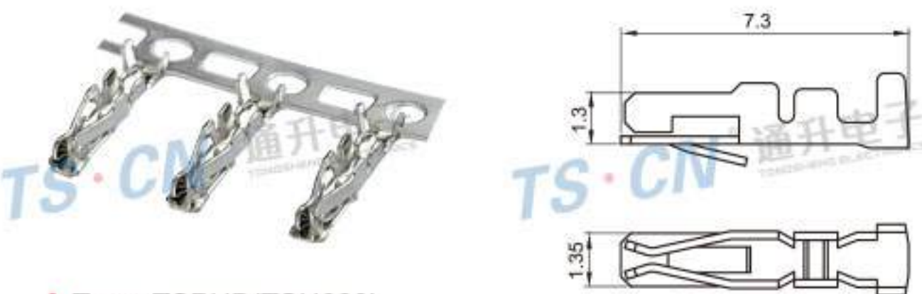
Type: TSPHB(TSH623) Material: Phos.bronze Applicable Thickness: 0.5
