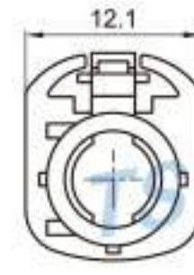
Type: TSVW20-04PF-AT-5BN Material: PA66 GF30% Matching Terminal: TSTF0048 / TSTF0049 / TSTF0050
