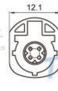
Type: TSVW10-04PM-AT-5BK Material: PA66 GF30% Matching Terminal: TSPM0021~TSPM0025
