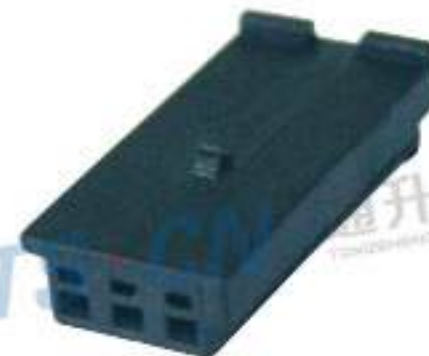
Type: TSBM03-03P-21-1 Material: PA66 GF15% Matching Terminal: TSH143
