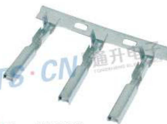
Type: TSH047 Material: Phos.bronze Applicable Thickness: 0.6~0.8
