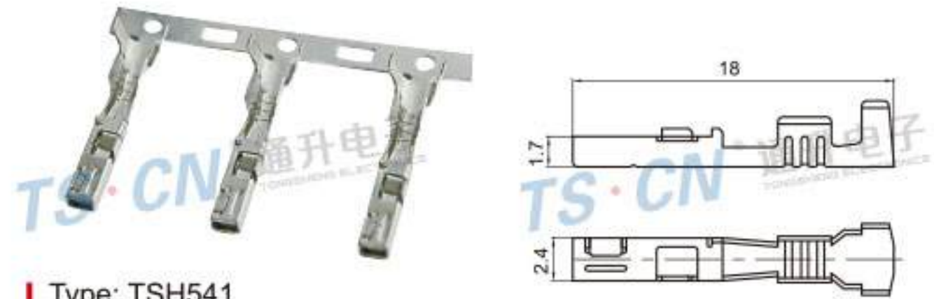
Type: TSH541 Material: Phos.bronze Applicable Thickness: 0.6
