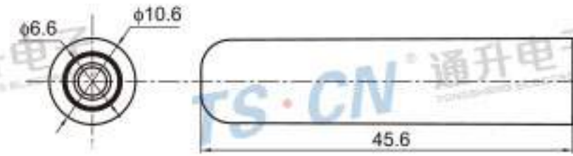
Type: TSHDAF-AT Material: PA6 Matching Terminal: TSTM0026 / TSTF0038
