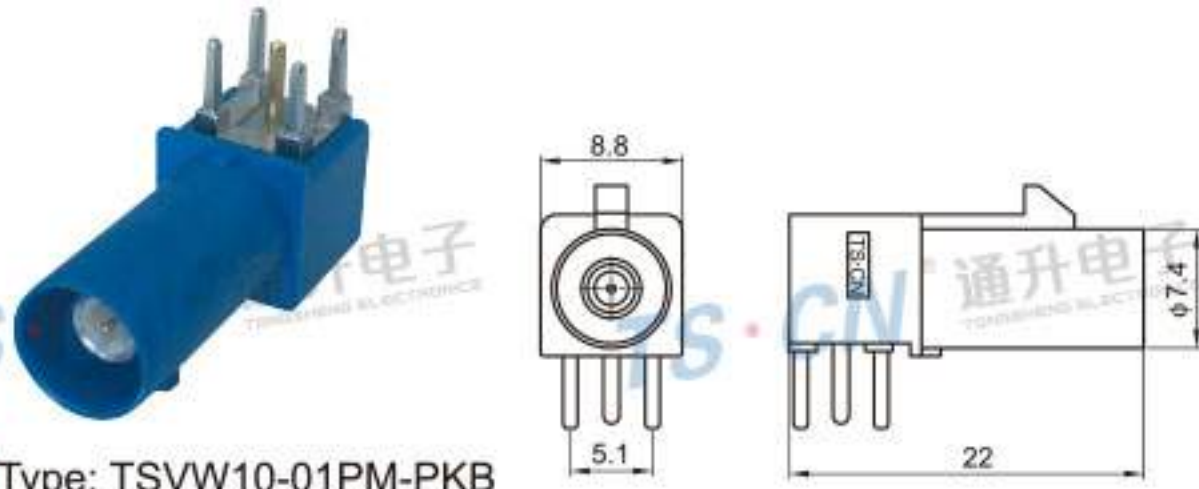
Type: TSVW10-01PM-PKB Material: PBT GF15% Matching Terminal: TSPM0169~TSPM0172
