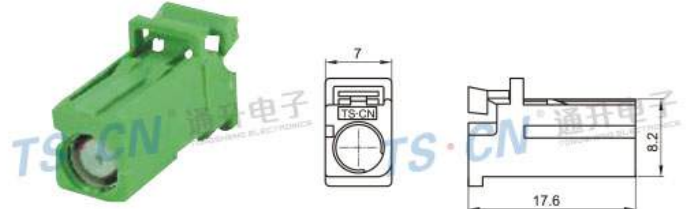
Type: TSGT16-01PF-AT-2 Material: PA66 Matching Terminal: TSTF0017 / TSTF0004
