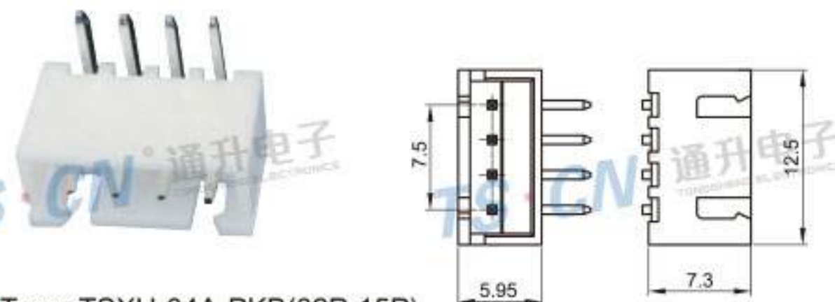
Type: TSXH-04A-PKB(02P-15P) Material: PA66 GF30% Matching Terminal: TSPM0299
