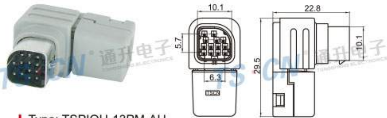
Type: TSPIOH-13PM-AH Material: PA66 Matching Terminal: TSAF0011 / TSAM0012 / TS0079
