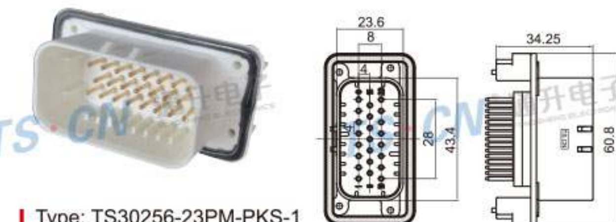
Type: TS30256-23PM-PKS Material: PBT GF30% Matching Terminal: TSPM0304
