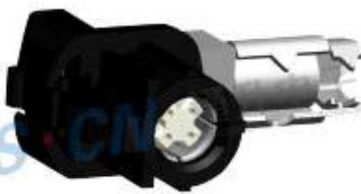
Type: TSVW20-04PF-AT-5BK Material: PA66 GF30% Matching Terminal: TSTF0048 / TSTF0049 / TSTF0050
