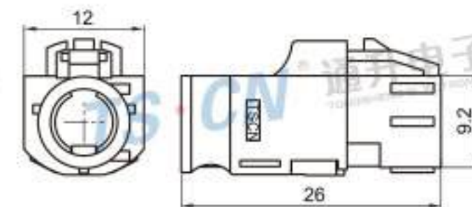
Type: TSVW20-04PF-AT-5YG-1 Material: PA66 GF30% Matching Terminal: TSTF0051 / TSTF0052
