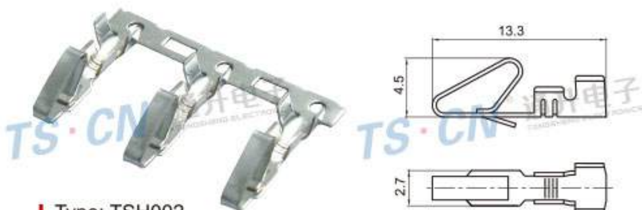
Type: TSH002 Material: Phos.bronze Applicable Thickness: 0.6~0.8
