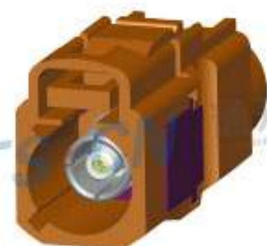
Type: TSVW20-01PF-AT-BN Material: PA66 GF30% Matching Terminal: TSTF0025 / TSTF0026
