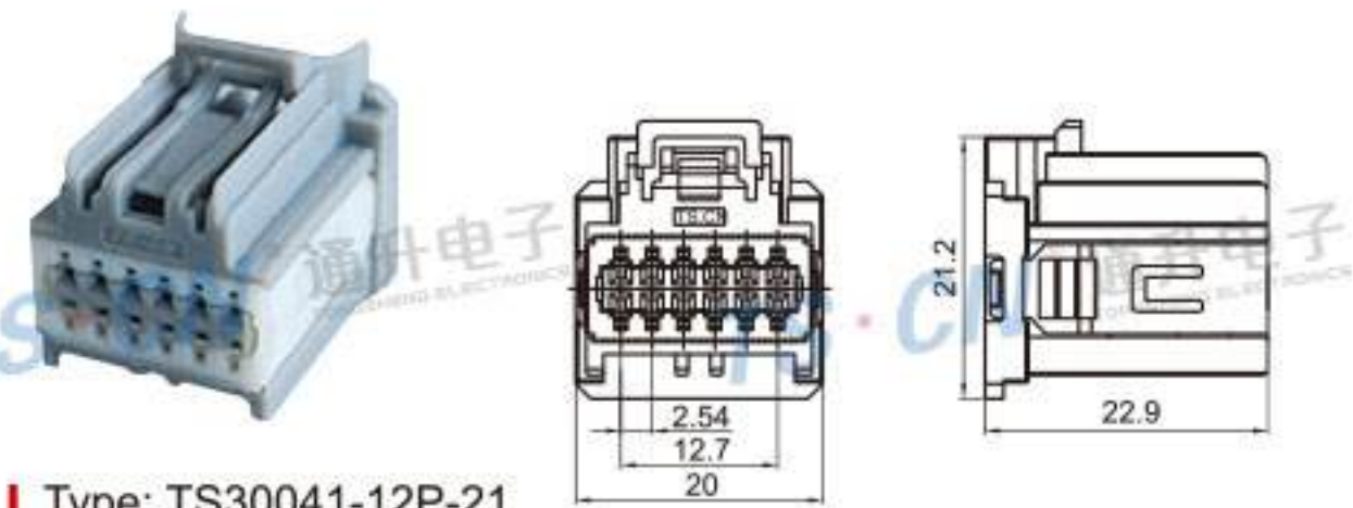
Type: TS30041-12P-21 Material: PA66 GF30% Matching Terminal: TSH006
