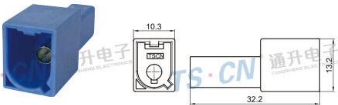
Type: TS1068-01PM-AT-1 Material: PA66 GF30% Matching Terminal: TSTM0003 / TSTM0004
