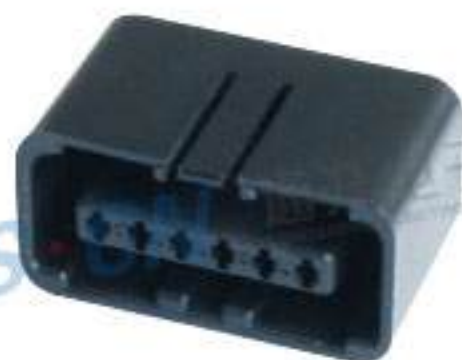
Type: TSGM06-06P-21 Material: PA66 GF15% Matching Terminal: TSH054
