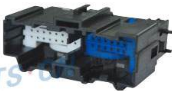
Type: TS2105-30P-11 Material: PA66 GF30% Matching Terminal: TSZ531 / TSZ530
