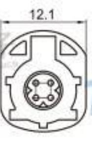
Type: TSVW10-04PM-AT-5CU Material: PA66 GF30% Matching Terminal: TSPM0021~TSPM0025
