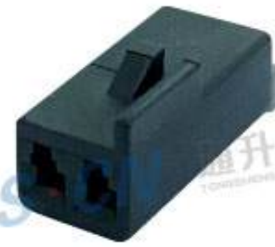
Type: TS30128-02P-21 Material: PA66 Matching Terminal: TSH639
