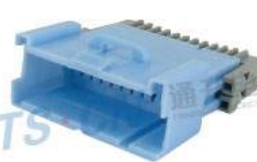
Type: TS2102-24P-11 Material: PA66 Matching Terminal: TSZ013
