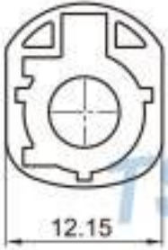
Type: TSVW10-04PM-AT-5YG-1 Material: PA66 GF15% Matching Terminal: TSPM0175 / TSTM0051
