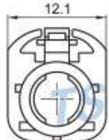
Type: TSVW20-04PF-AT-5CU Material: PA66 GF30% Matching Terminal: TSTF0048 / TSTF0049 / TSTF0050
