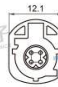
Type: TSVW10-04PM-AT-5BE Material: PA66 GF30% Matching Terminal: TSPM0021~TSPM0025
