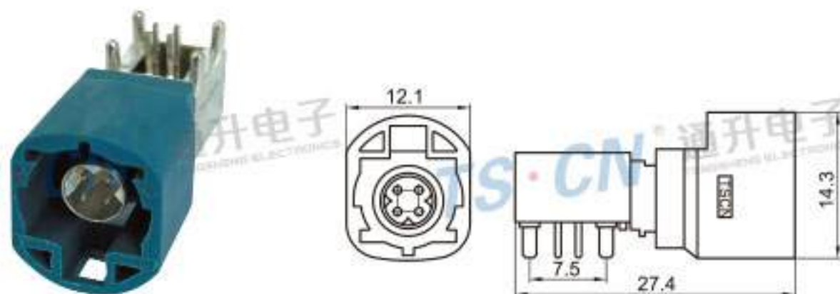
Type: TSVW10-04PM-AT-5WB Material: PA66 GF30% Matching Terminal: TSPM0021~TSPM0025
