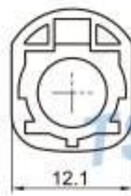
Type: TSVW10-04PM-AT-5WB-1 Material: PA66 GF15% Matching Terminal: TSPM0175 / TSTM0051
