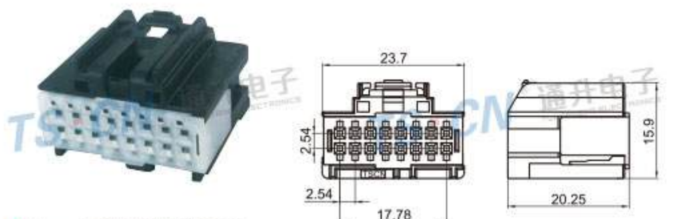
Type: TS30244-16P-21 Material: PBT Matching Terminal: TSH006
