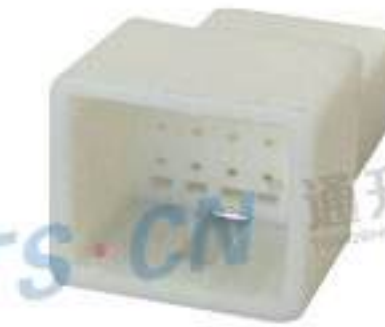
Type: TS30037-10P-11 Material: PA66 Matching Terminal: TSZ208B
