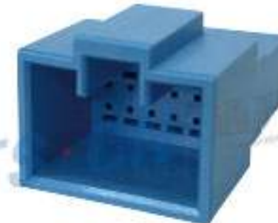
Type: TS30296-12P-11 Material: PBT GF15% Matching Terminal: TSZ616
