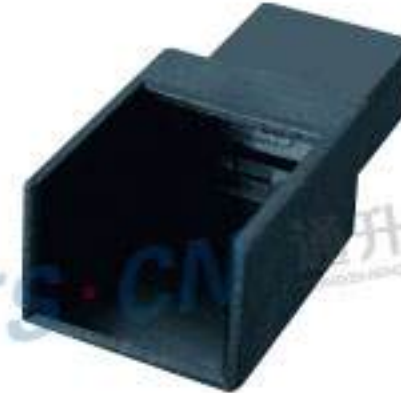
Type: TS30181-01P-11 Material: PA66 GF30% Matching Terminal: TSZ613
