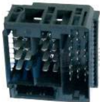
Type: TSVW36-36PM-PKS-1 Material: PA66 GF30% Matching Terminal: TSPM0109~TSPM0113
