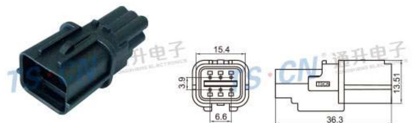
Type: TS30207-06P-11 Material: PBT GF15% Matching Terminal: TSZ537
