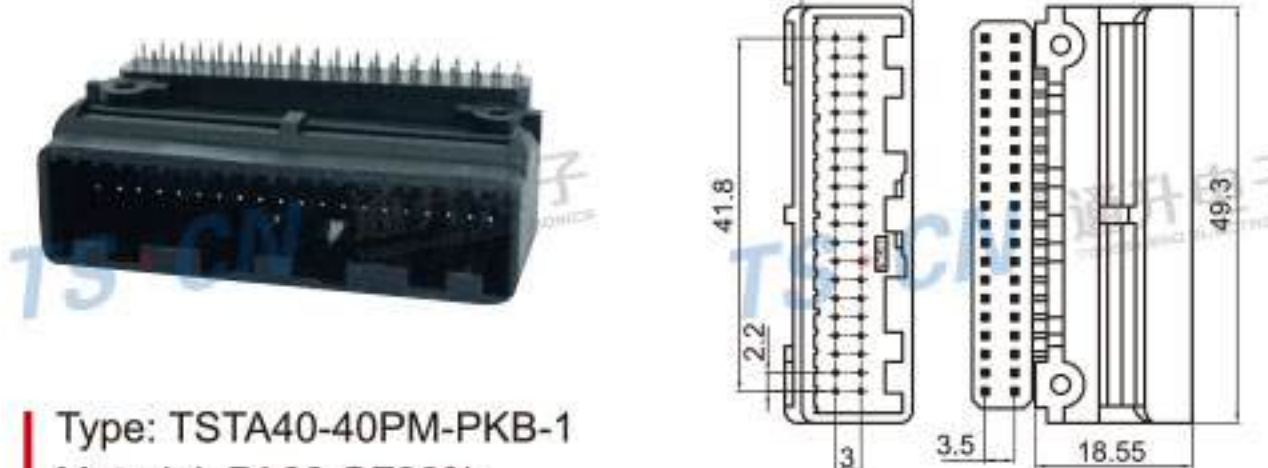
Type: TSTA40-40PM-PKB Material: PBT GF15% Matching Terminal: TSPM0040/TSPM0041
