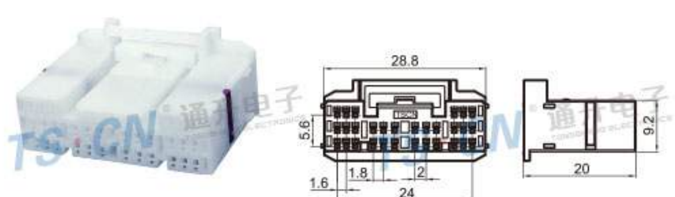
Type: TS30101-30P-21-5 Material: PA66 Matching Terminal: TSH600A
