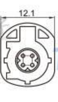
Type: TSVW10-04PM-AT-5GN Material: PA66 GF30% Matching Terminal: TSPM0021~TSPM0025
