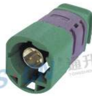
Type: TSVW10-04PM-AT-5GN-1 Material: PA66 GF15% Matching Terminal: TSPM0175 / TSTM0051
