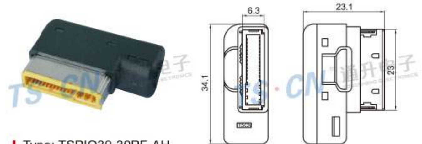
Type: TSPIO30-30PF-AH Material: PA66 GF15% Matching Terminal: TSAF0005 / TSAF0006 / TSAF0008
