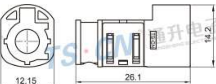
Type: TSVW10-04PM-AT-5BN-1 Material: PA66 GF15% Matching Terminal: TSPM0175 / TSTM0051
