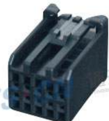
Type: TSGM10-10P-21 Material: PA66 GF30% Matching Terminal: TSH143
