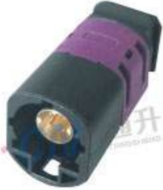
Type: TSVW10-04PM-AT-5BK-1 Material: PA66 GF15% Matching Terminal: TSPM0175 / TSTM0051
