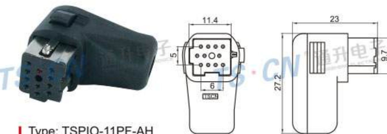
Type: TSPIO-11PF-AH Material: PA66 GF30% Matching Terminal: TSAF0009 / TSAF0010 / TSH501
