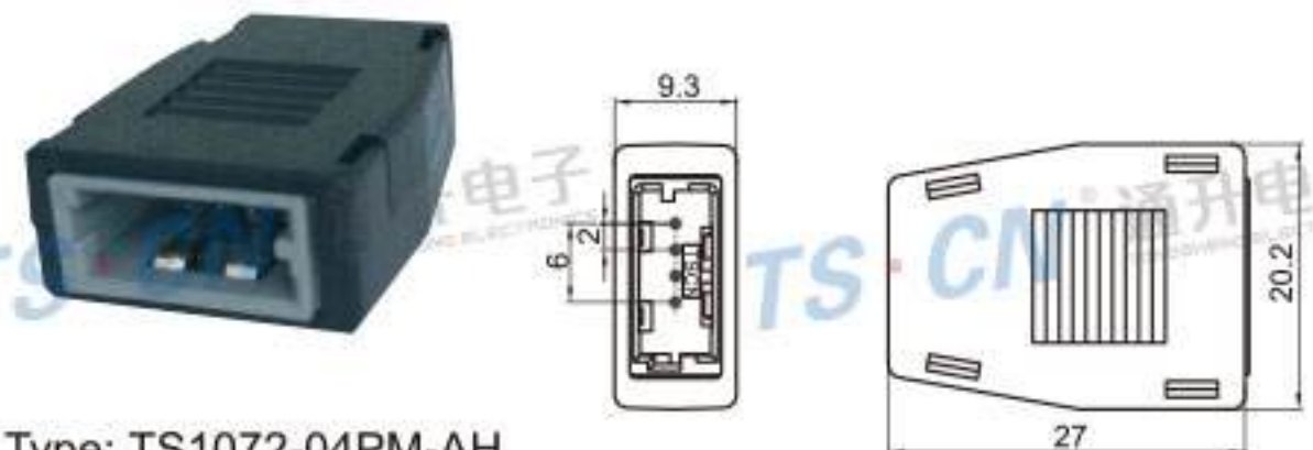
Type: TS1072-04PM-AH Material: ABS Matching Terminal: TSPM0237 / TSPM0030
