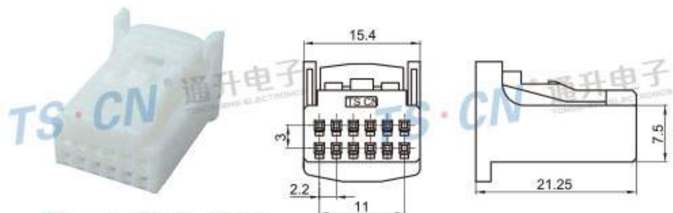
Type: TSTA12-12P-21 Material: PA66 Matching Terminal: TSH143
