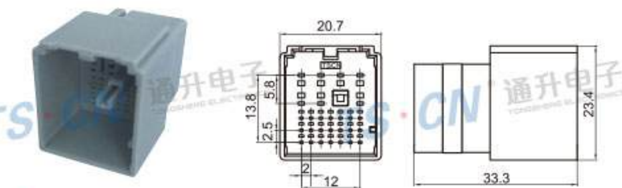
Type: TS30205-28P-11-1 Material: PA66 Matching Terminal: TSZ566 / TSZ561
