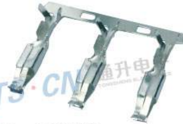
Type: TSH019C Material: Phos.bronze Applicable Thickness: 0.5~0.8
