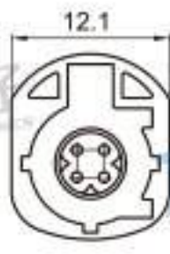
Type: TSVW10-04PM-AT-5BN Material: PA66 GF30% Matching Terminal: TSPM0021~TSPM0025
