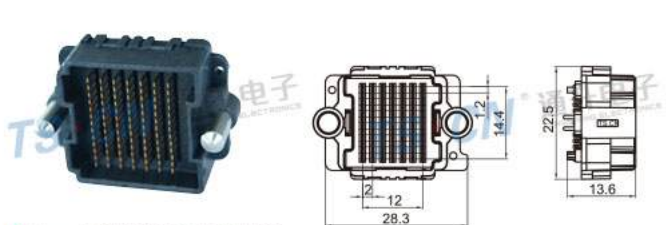
Type: TS30034-91PM-PKS Material: LCP GF30% Matching Terminal: TSPM0200 / TSPM0201
