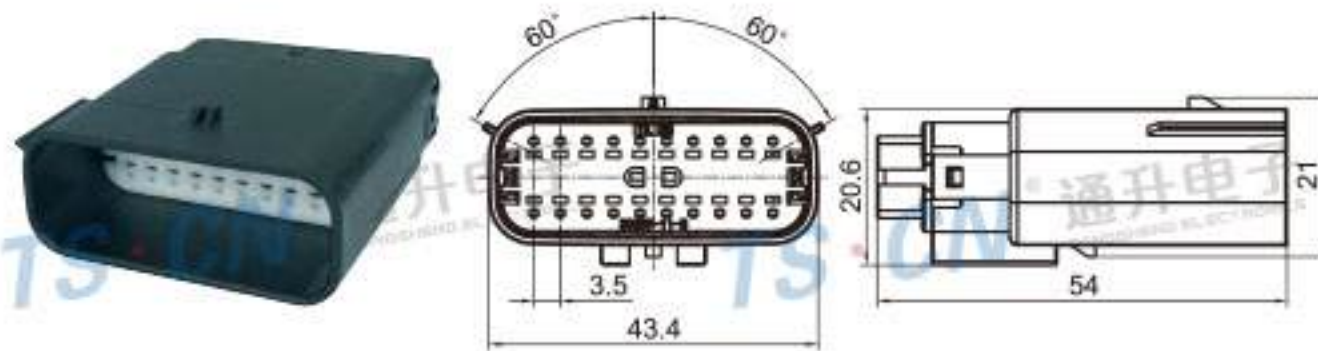
Type: TS30359-20P-11 Material: PA66 GF30% Matching Terminal: TSZ144A
