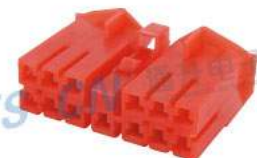
Type: TSCIT-13P-21 Material: PA66 Matching Terminal: TSH012
