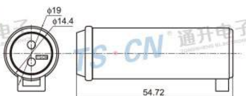
Type: TSNI01-02PM-AT Material: ABS Matching Terminal: TSTM0025 / TSTM0026
