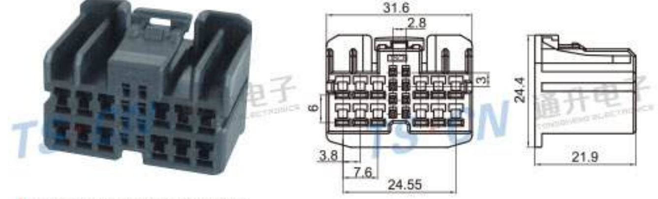
Type: TS30071-20P-21 Material: PA66 GF30% Matching Terminal: TSH009 / TSH143
