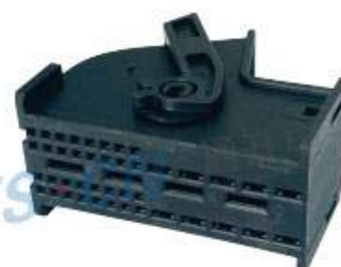
Type: TSBM42-42P-21-2 Material: PA66 GF30% Matching Terminal: TSH091 / TSH143
