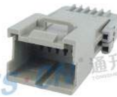
Type: TS2012-12P-11 Material: PA66 Matching Terminal: TSZ013
