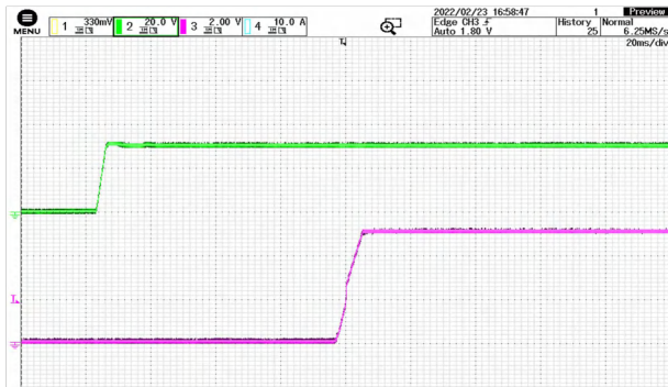
Figure 6 Start waveform @ VIN=30V CH2: VIN CH3: Vout
