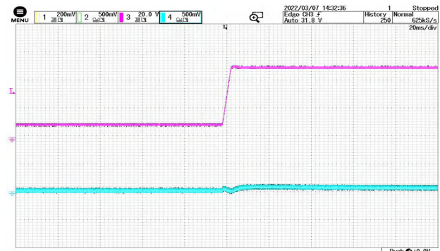
Figure 11 9V-50V Input Jump @ 10% Load CH3: VIN CH4: Vout
