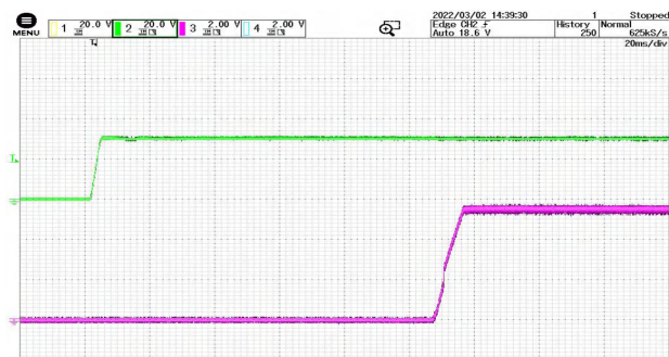
Figure 13 Output Upregulation CH2:VIN CH3:Vout Start Waveform @ VIN=30V
