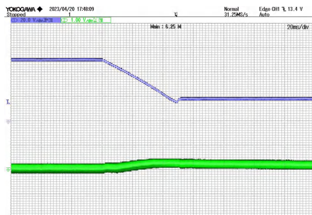
Figure 10 50V-16V Input Jump @ 10% Load CH1: VIN CH2: Vout
