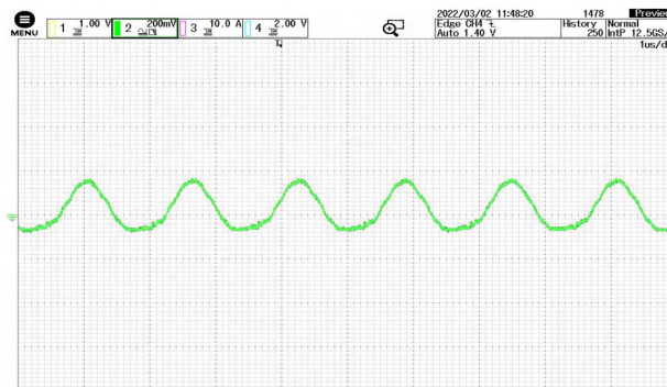
Figure 7 Output voltage ripple @ VIN=28V at full load
