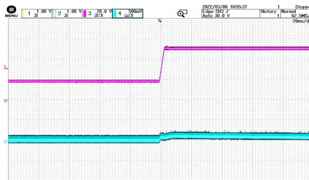
Figure 11 16V-50V Input Jump @ 10% Load CH3: VIN CH4: Vout
