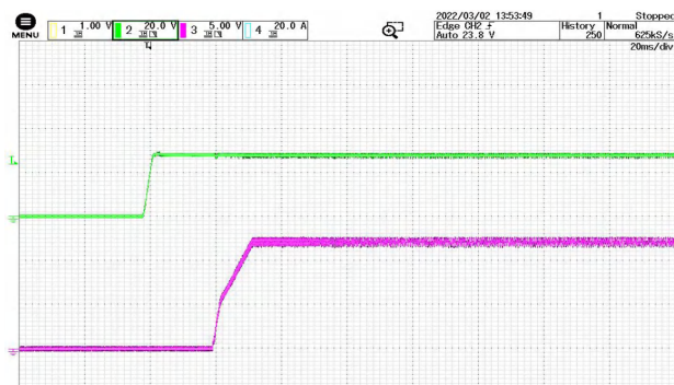
Figure 6 Start waveform @ VIN=28V CH2: VIN CH3: Vout
