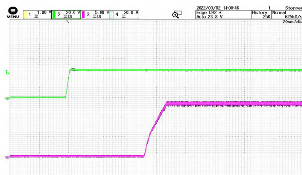
Figure 13 Output Upregulation CH2:VIN CH3:Vout Start Waveform @ VIN=28V
