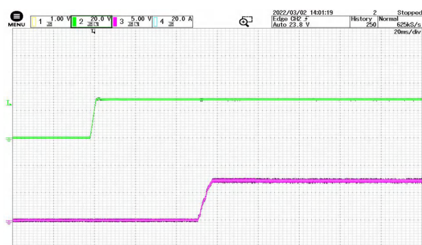
Figure 12 Output Downregulation CH2:VIN CH3:Vout Start Waveform @ VIN=28V
