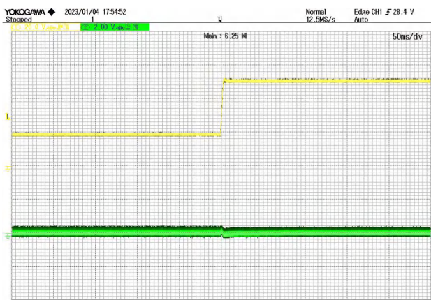
Mean(C1) 35.3061 V Mean(C2) 42.9757mV Acquire 50ms/div, 12.5MS/s, 6.25MPoints, Normal Trigger Edge CH1 F 28.4 V, Auto CH1 CH2 100:1 10:1 20.0 V/div 2.00 V/div DC1M0 1M AC1M0 20M Figure 11 16V-50V Input Jump CH1: V_{IN} CH2: V_{out} @ 10% Load
