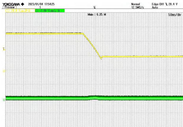
Mean(C1) 34.7521 V Mean(C2) 54.2566mV Acquire 50ms/div, 12.5MS/s, 6.25MPoints, Normal Trigger Edge CH1 F 28.4 V, Auto CH1 CH2 100:1 10:1 20.0 V/div 2.00 V/div DC1M0 1M AC1M0 20M Figure 10 50V-16V Input Jump CH1: V_{IN} CH2: V_{out} @ 10% Load
