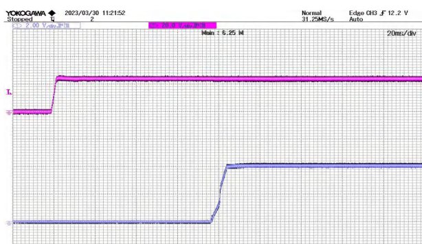
Figure 12 Output Downregulation Start Waveform @ VIN=24V CH1:VIN CH2:V out
