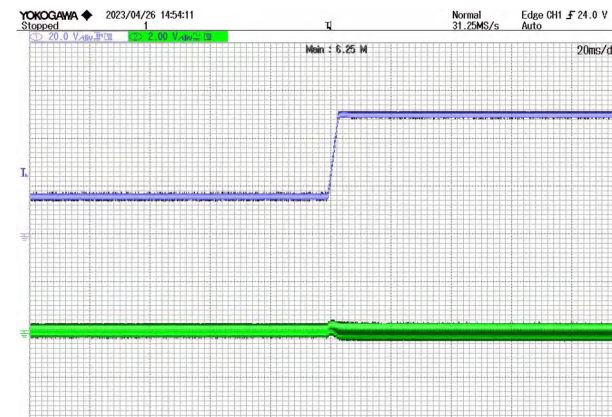
Figure 11 16V-50V Input Jump @ 10% Load CH1: VIN CH2: Vout
