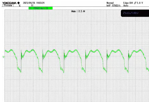
Figure 7 Output voltage ripple @ VIN=28V at full load
