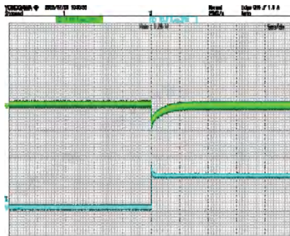
Figure 9 10% load -90% load jump @ VIN=30V CH2: Vout CH4: Io
