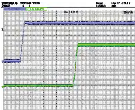
Figure 6 Start waveform @ VIN=30V CH2: VIN CH3: Vout
