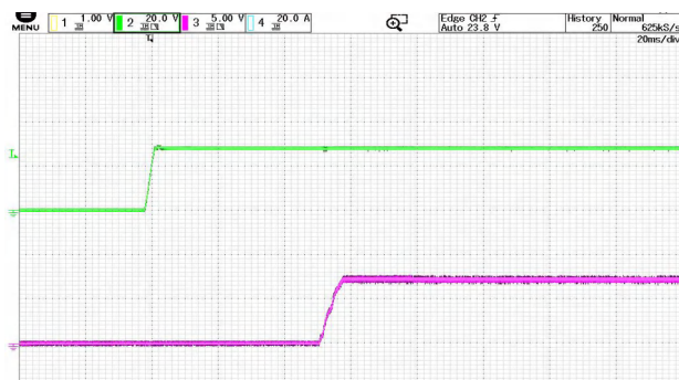
Figure 12 Output Downregulation Start Waveform @ VIN=30V CH2:VIN CH3:Vout
