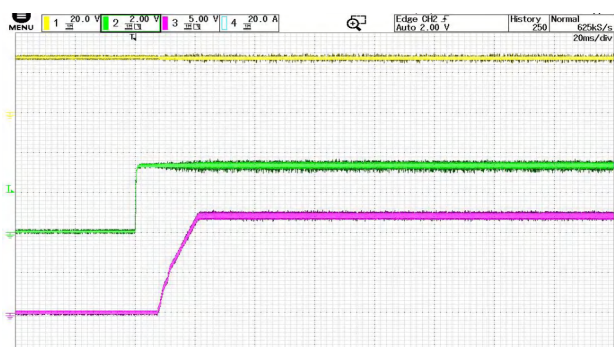
Figure 14 Start waveform (enabled) @ VIN=30V CH1:VIN CH2: EN CH3:Vout
