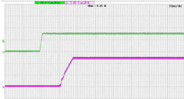
Figure 6 Start waveform @ VIN=30V CH2: VIN CH3: Vout
