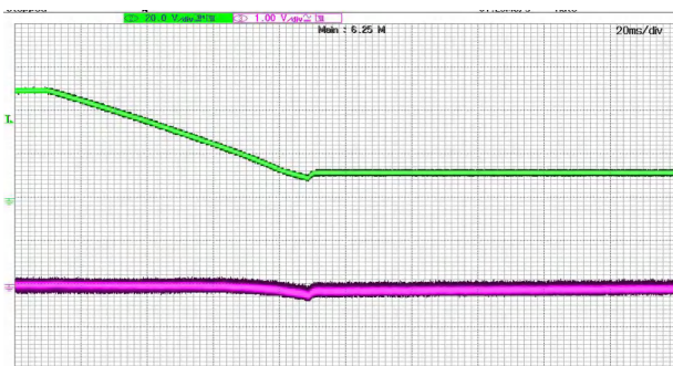
Figure 10 50V-9V Input Jump @ 10% Load CH2: VIN CH3: Vout
