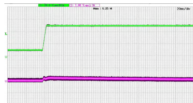
Figure 11 9V-50V Input Jump @ 10% Load CH2: VIN CH3: Vout
