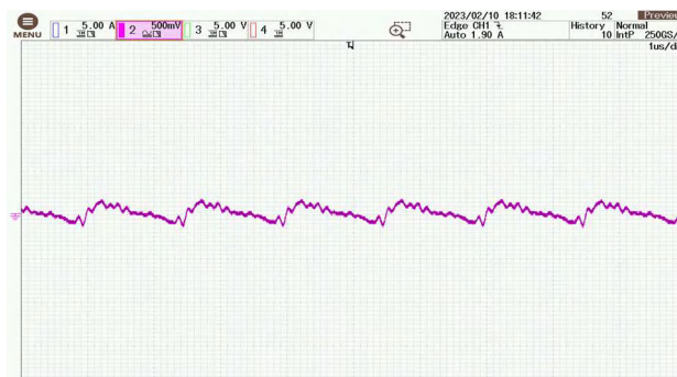
Figure 7 Output voltage ripple @ VIN=30V at full load
